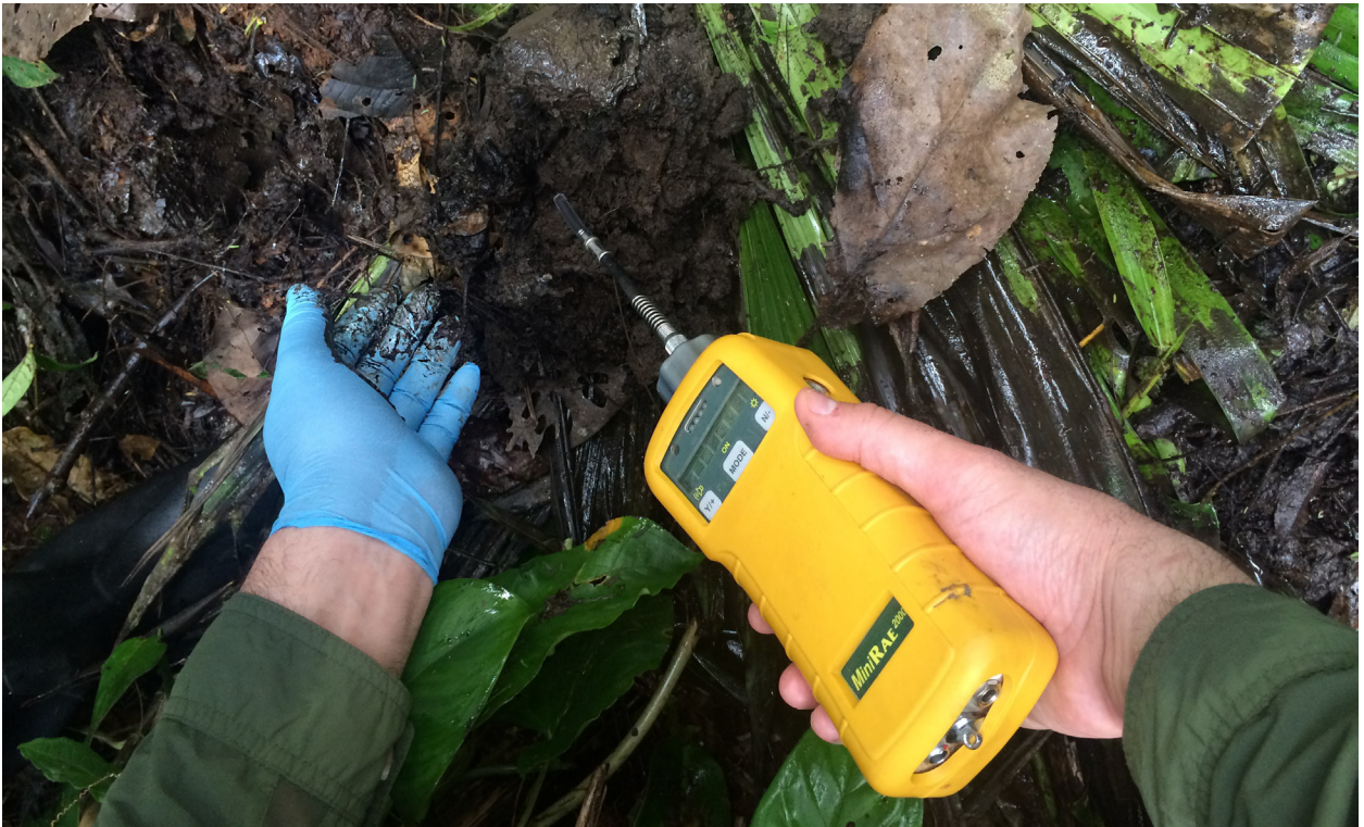
Shushufindi 55, April 2015, detecting device for volatile organic compounds used to measure the pollution levels.
